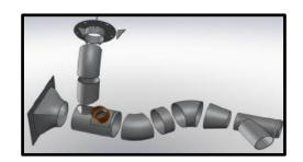
**Traditional Part:** 19 aluminum parts welded together
